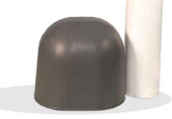
Install the shell vent with the open end facing downward, ideally at a 45° angle, for optimal airflow. Use a 1-1/4" PVC pipe for secure hose adapter fitting.
